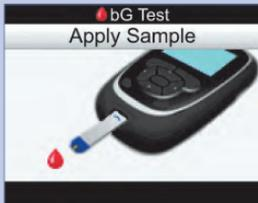
The Apply Sample screen is displayed. Place the meter on a flat surface.
