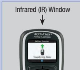
Locate the infrared (IR) window on the top of the meter.
