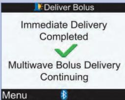
The meter displays this screen when the immediate bolus amount has been delivered.
