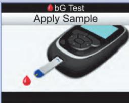
The Apply Sample screen is displayed. Perform a fingerstick with the aid of a finger pricker.
