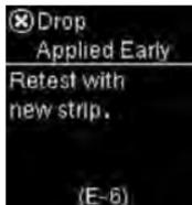
Blood or control solution was applied to the test strip before **Apply drop** appeared.
