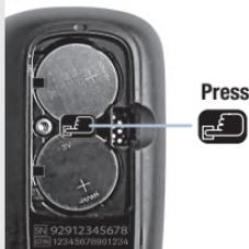
Release the old batteries by pressing the
