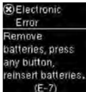
An electronic error occurred. Remove the batteries, press and hold the Power/Set/OK button for at least 2 seconds, and reinsert the batteries. Perform a blood glucose or control test.
