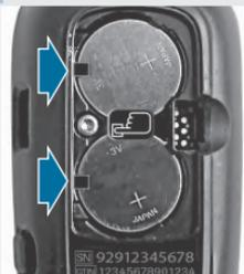
Slide the new batteries under the black tabs and
