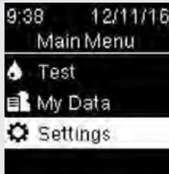
Turn the meter on by briefly pressing **OK**. From **Main Menu**, press **▼** to highlight **Settings**. Press **OK**.
