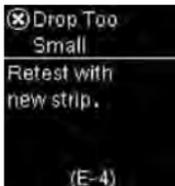
Not enough blood or control solution was drawn into the test strip for measurement or was applied after the test had started.
