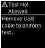
The meter is connected to a USB cable and a test cannot be performed.
