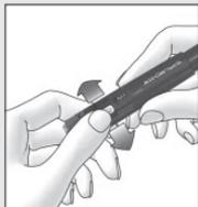
Load the next lancet by sliding the lever (until it stops), then slide it back all the way.
