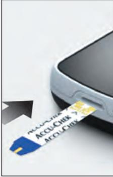
Insert the test strip into the meter in the direction of the arrows. The meter turns on.
