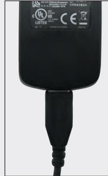
Plug the larger end of the USB cable into the power adapter.
