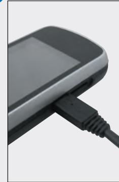
Plug the smaller end of the USB cable into the meter.
