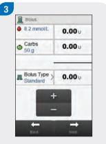
Enter the bolus amounts, as necessary. To input a bolus amount, select the entry field for Correction Bolus, Carbohydrate Bolus or Total Bolus and set the amount.
