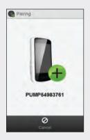
The meter attempts to pair with the pump and displays the Pairing screen.
