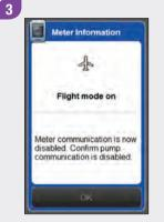
Select OK. Communication on both the meter and pump is disabled. Confirm that the symbol appears on the pump.
