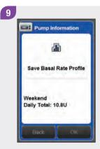
Select OK. The meter saves the changes to the basal profile.
