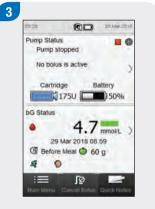
The meter displays the Status screen, which shows that the pump has stopped.
