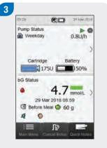
The meter displays the Status screen, which shows that the pump has started.
