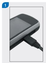
Plug the smaller end of the USB cable into the meter.
