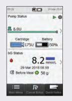
The pump delivers the bolus and the meter displays the Status screen showing the current bolus information.
