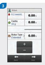
Enter the bolus amounts as necessary. To input the bolus amount, select the entry field for Correction Bolus, Carbohydrate Bolus or Total Bolus, and set the amount.
