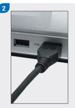
Plug the larger end of the USB cable into an available USB port on the PC. If the battery is extremely low on power, the meter does not turn on. Charge the battery using a power outlet.
