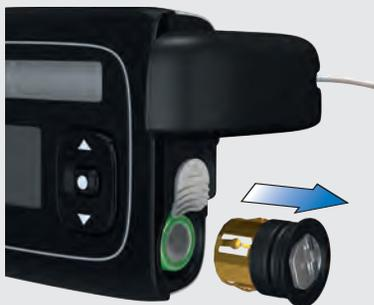
Remove the battery cover and the old battery.
