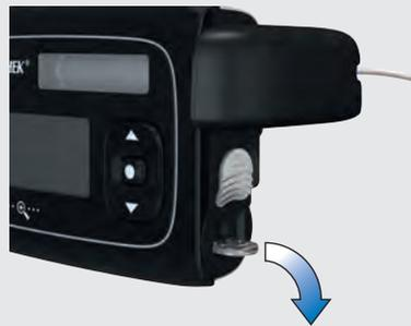
You can use the flip-up handle to easily remove the battery cover.
