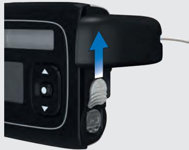
Push the battery cover release in the direction of the arrow (towards the cartridge compartment).
