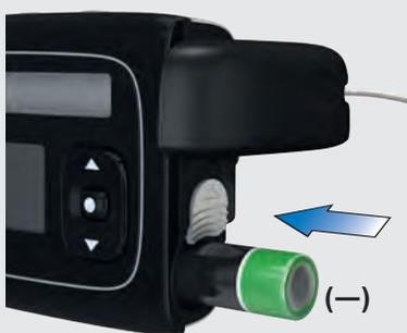
Insert the new battery into the battery compartment, positive (+) end first, negative (-) end pointing outwards.
