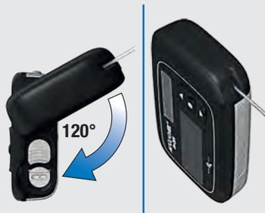
Turn the adapter clockwise all the way until it stops. The adapter is correctly positioned when it is aligned with the pump's housing.
