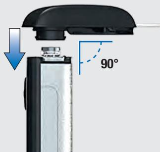
Place a **new adapter** on the bayonet socket of the cartridge compartment. Make sure you insert the nose of the adapter into the notches of the pump's housing at a right angle (90°). Otherwise the needle could bend.
