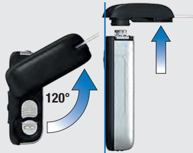
When you reach an angle of 120°, remove the adapter with the cartridge. The pump starts rewinding the piston rod.
