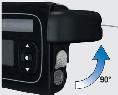
Turn the adapter anti-clockwise to a 90° position.
