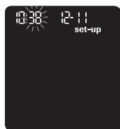
2. Press and hold down ▼ until set-up appears on the display. The hour flashes. Press up ▲ to increase the hour or press down ▼ to decrease the hour.
