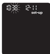
3. Press and hold up ▲ to set the hour and move to the next field. The minutes flash. Press up ▲ to increase the minutes or press down ▼ to decrease the minutes.
