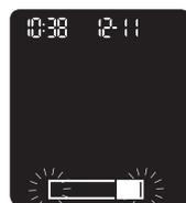
4. Repeat step 3 to adjust each field. After setting the year, press and hold up ▲ until the flashing test strip symbol appears to save your settings.
