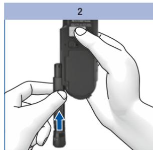
Slide the finger pricker along the side of the meter in the direction of the arrow until it slots into place.
