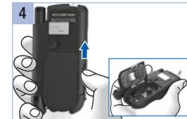
Push the slide button for the cassette compartment cover upwards in the direction of the arrow.
