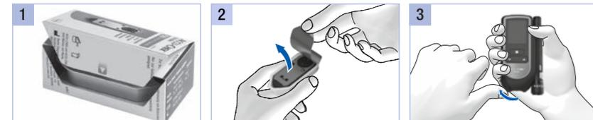
Open the test cassette box at the perforation. Take out the plastic container.
