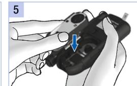
Insert the test cassette in the meter. Press the cassette compartment cover closed. Close the tip cover.
