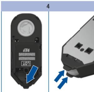
Check whether you can see any dirt inside the tip of the cassette. If so, remove this carefully.
