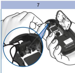
Carefully dab the interior of the tip cover with a slightly dampened cotton swab.
