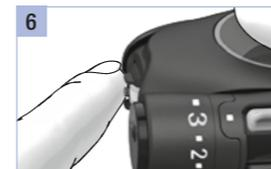
To apply the blood drop to the test area: Position your finger gently on the guidance tabs so that **only** the blood drop comes into contact with the test area between the guidance tabs.
