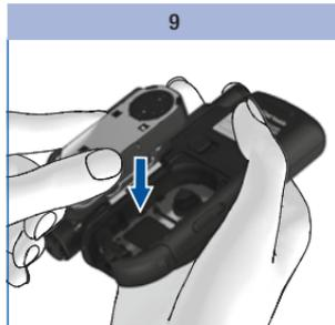
Re-insert the test cassette in the meter.
