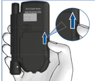
Push the slide button for the cassette compartment cover upwards.
