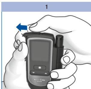
Push the battery door in the direction of the arrow as far as it will go to open it.
