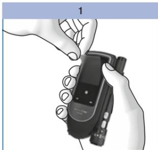
Remove the protective film from the display.
