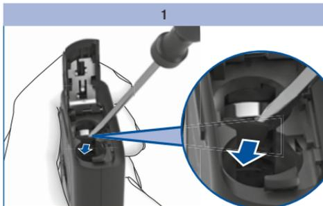
Use a small screwdriver to break out the partition wall in front of the battery.
