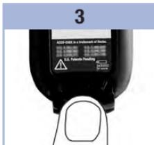
Slide the battery drawer back into position until it locks into place. The meter prompts you for a time and date confirmation when it is turned on.
