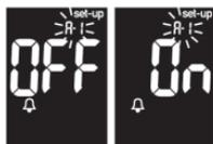
Press and release
