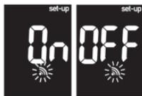
Press and release
