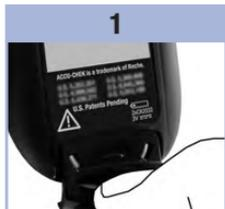
Use your thumb to slide the battery drawer out of the meter.
