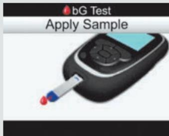
The Apply Sample screen appears. The test strip is ready for testing.
