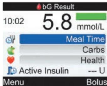
The detailed bG Result screen allows you to view and to add information to a blood glucose test result.
